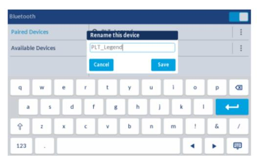
5. Edit the name of the device using the on-screen keyboard tap the **Save** softkey to save your changes.
