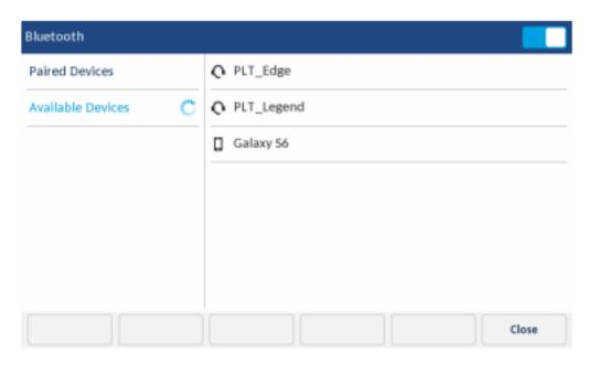
NOTE: The Mitel MiVoice 6940 IP phone scans for supported Bluetooth devices when viewing the list of available devices. Refer to the respective Bluetooth device documentation for discovery and pairing procedures that must be performed on your Bluetooth device.
