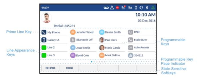
If you have 16 or more programmable keys configured, programmable page indicators are displayed at the bottom of the screen. These dots indicate the number of programmable key pages and its relative position. Swipe left and right on the programmable key area to switch the programmable key pages.
