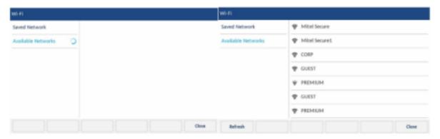
4. Select an SSID (that is, the name of a Wi-Fi network, for example, **Mitel Secure**) from **Available Networks**to connect. If the SSID is secured, a password prompt appears.
