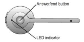
3. Dock the new headset in the base. The new headset is paired with the base after 1 minute.
