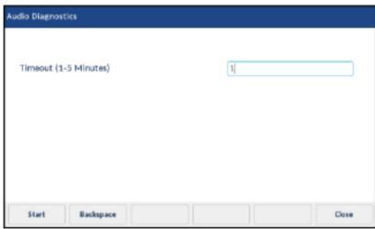
4. In the **Timeout** input field, enter the amount of time (in minutes from 1 to 5) you would like to run the audio diagnostic tool for using the dialpad keys.
