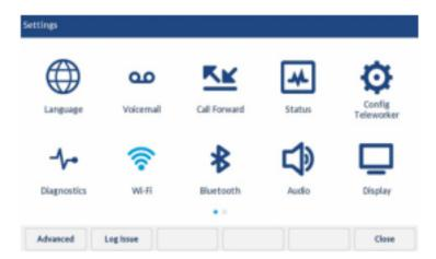
2. Ensure that a WLAN adapter is connected to the phone. The phone displays an error if it is not connected to a WLAN adapter.
