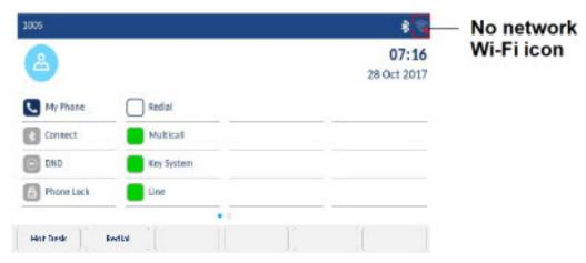
2. **Not Connected** - The phone is connected to the WLAN adapter but not connected to MiVoice Business or MiVoice Border Gateway.
